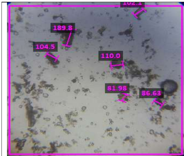
Figure 1: Microscopic Observation of Particle Size for the sample PUC
